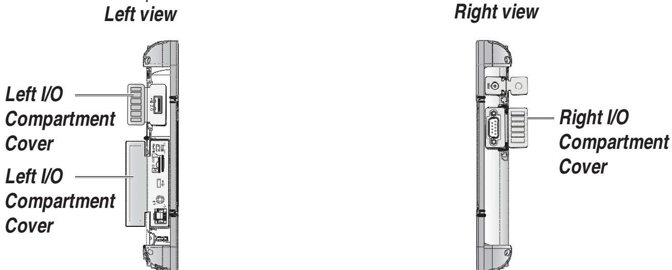
Figure 19. Side View: Locating the I/O Compartment Cover
