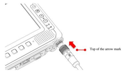
3. Twist the nut to lock the power connector to the device.
