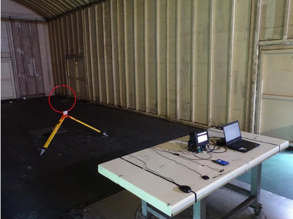
Front View of Radiated Test-LOOP
