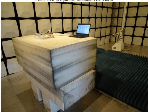
Front View of Spurious Emission Test (Horn)
