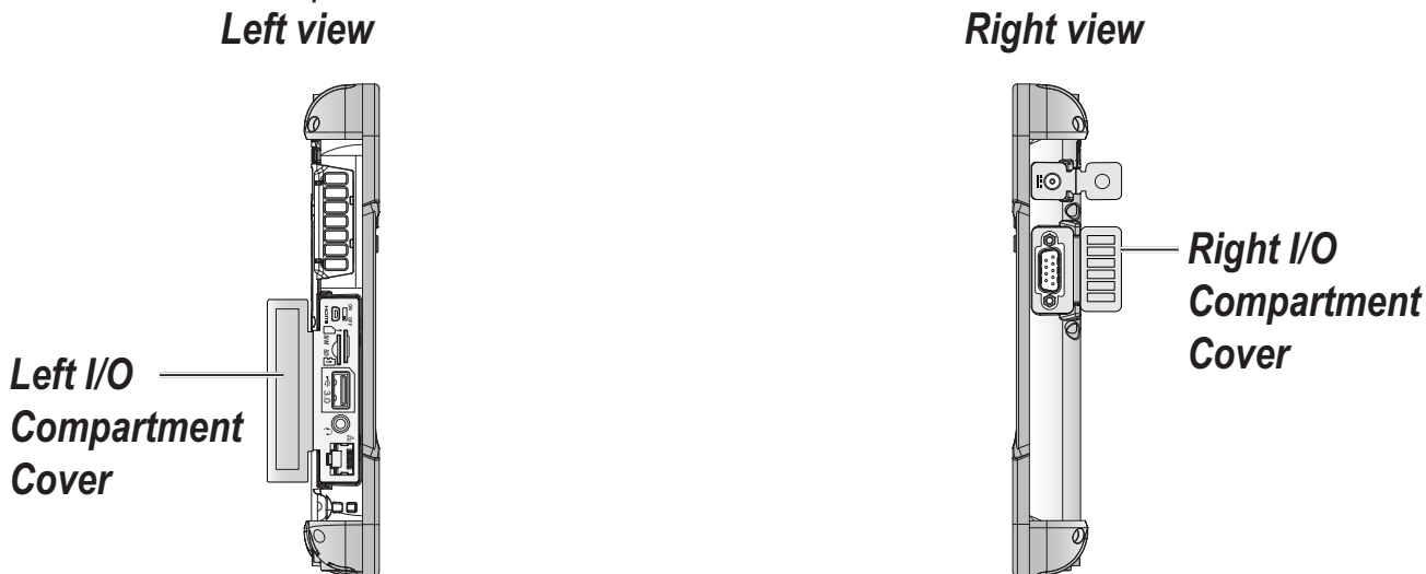
Figure 26. Side View: Locating the I/O Compartment Cover
