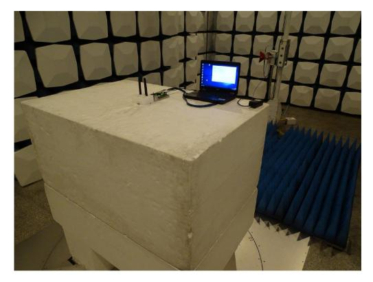
Front View of Radiated Test (Horn)
