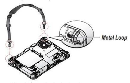
Figure 42. Connecting the Shoulder Strap
