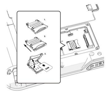
Figure 15. Installing the Micro SIM Card
