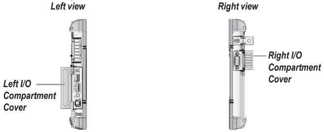
Figure 20. Side View: Locating the I/O Compartment Cover
