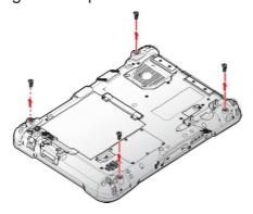
Figure 34. Removing the Screws
