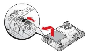
Figure 49. Removing the Battery
