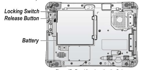
Figure 47. Rear View: Locating the Battery
