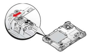
Figure 48. Unlock the Battery
