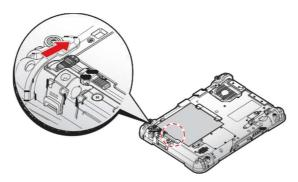
Figure 46. Locking the Battery
