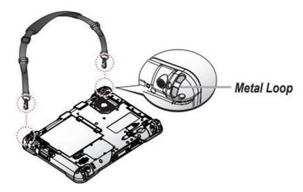
Figure 43. Removing the Shoulder Strap
