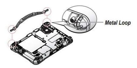
Figure 41. Removing the Carrying Handle
