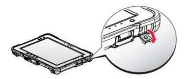
Figure 9. Opening the DC-IN Cover
