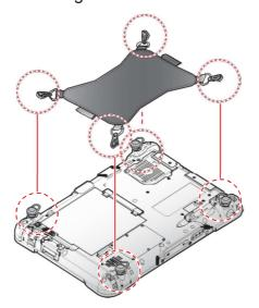
Figure 37. Removing the Handstrap
