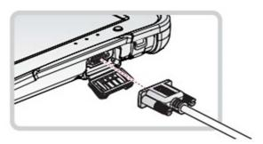
Figure 33. Connect RS-232 Cabling
