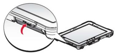
Figure 21. Installing the I/O Compartment Cover
