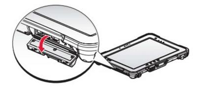
Figure 19. Opening the I/O Compartment Cover
