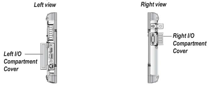
Figure 17. Side View: Locating the I/O Compartment Cover
