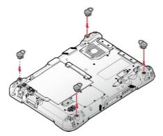
Figure 35. Installing the D-rings
