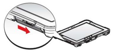
Figure 22. Locking the Latch
