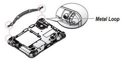
Figure 40. Connecting the Carrying Handle
