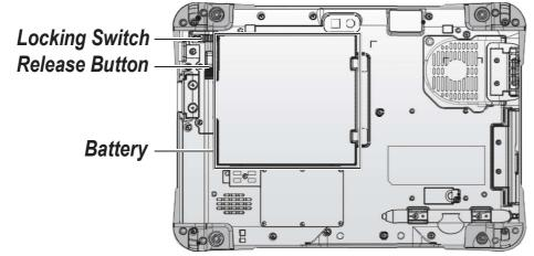
Figure 44. Rear View: Locating the Battery
