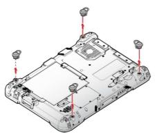
Figure 38. Removing the D-rings
