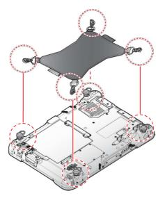
Figure 36. Connecting the Handstrap
