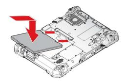
Figure 45. Installing the Battery
