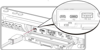
Figure 26. Connect Micro HDMI Cabling
