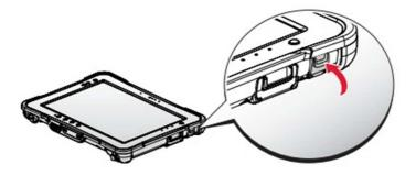
Figure 11. Closing the DC-IN Cover
