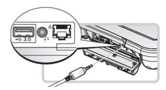
Figure 25. Connect Audio Cabling
