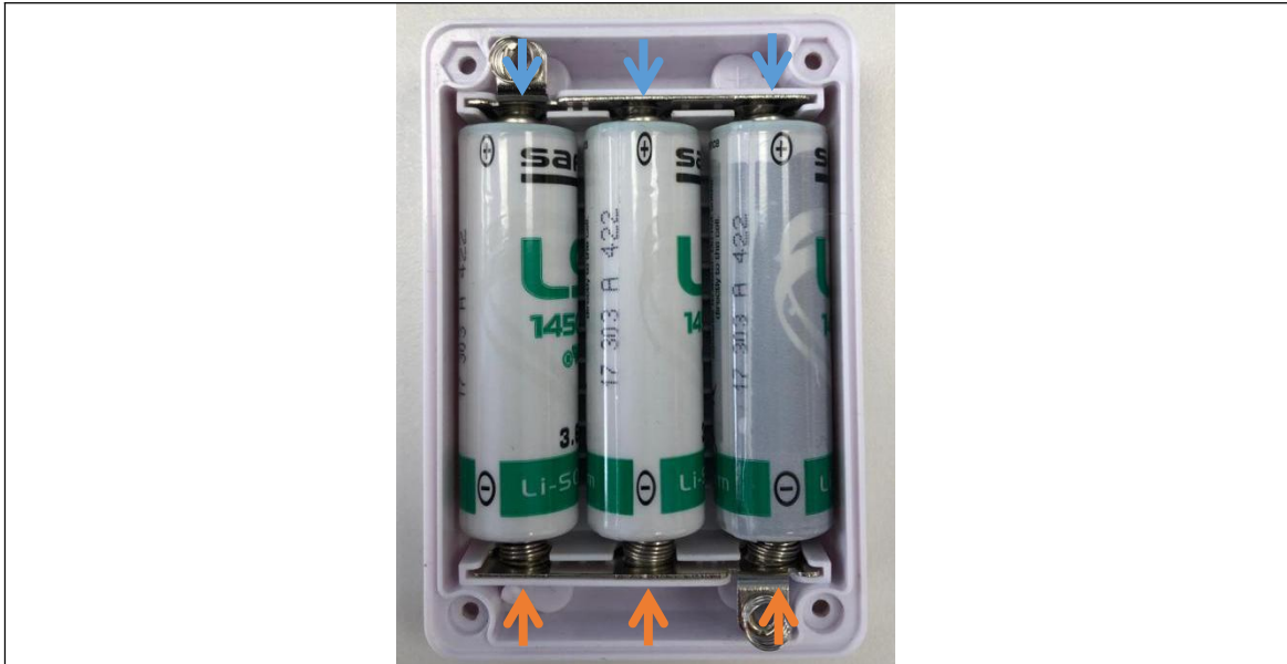
Figure 4 - TRK210 battery compartment with the batteries in the right position. Blue arrows mark positive pole and orange arrows mark negative pole.
