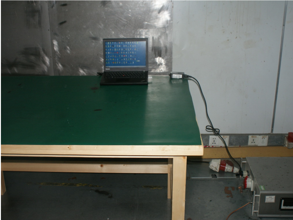
Photograph 6: Set-up for Radiated Emissions, below 1GHz
