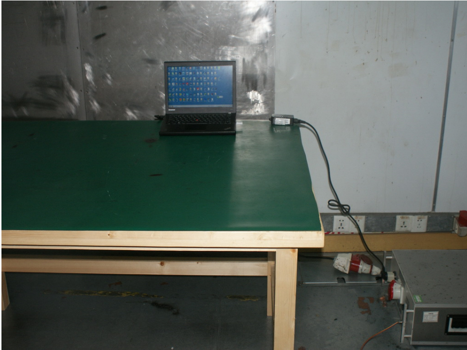
Photograph 6: Set-up for Radiated Emissions, below 1GHz
