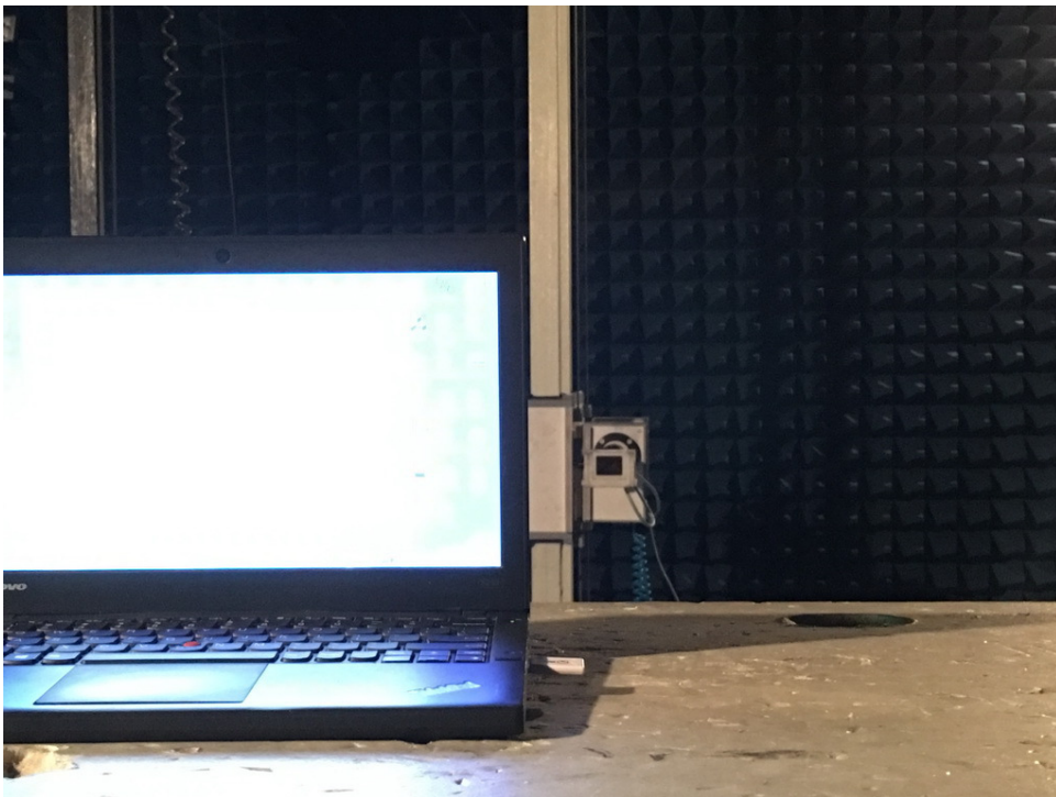
Photograph 4: Set-up for Spurious Emissions (18GHz-26GHz)
