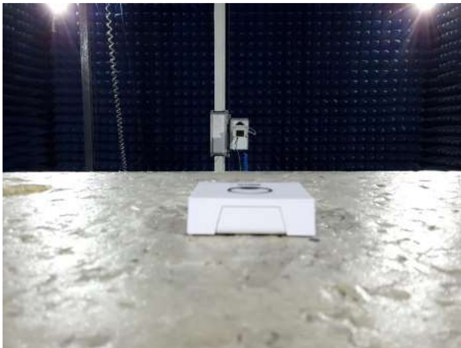
Photograph 4: Set-up for Radiated Spurious Emission above 18GHz
