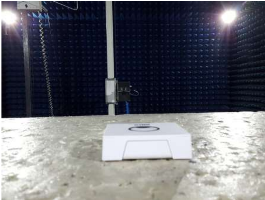
Photograph 3: Set-up for Radiated Spurious Emission (1GHz ~ 18GHz)
