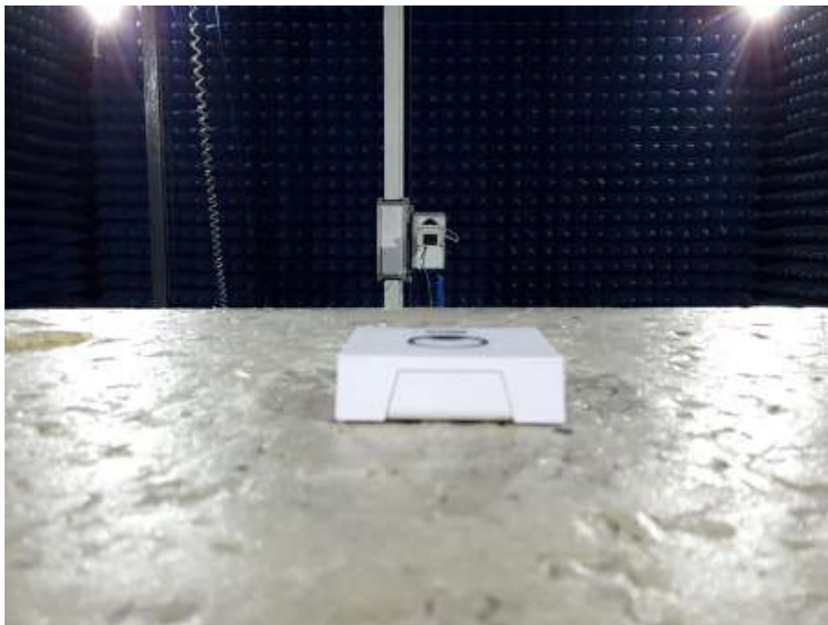
Photograph 4: Set-up for Radiated Spurious Emission above 18GHz
