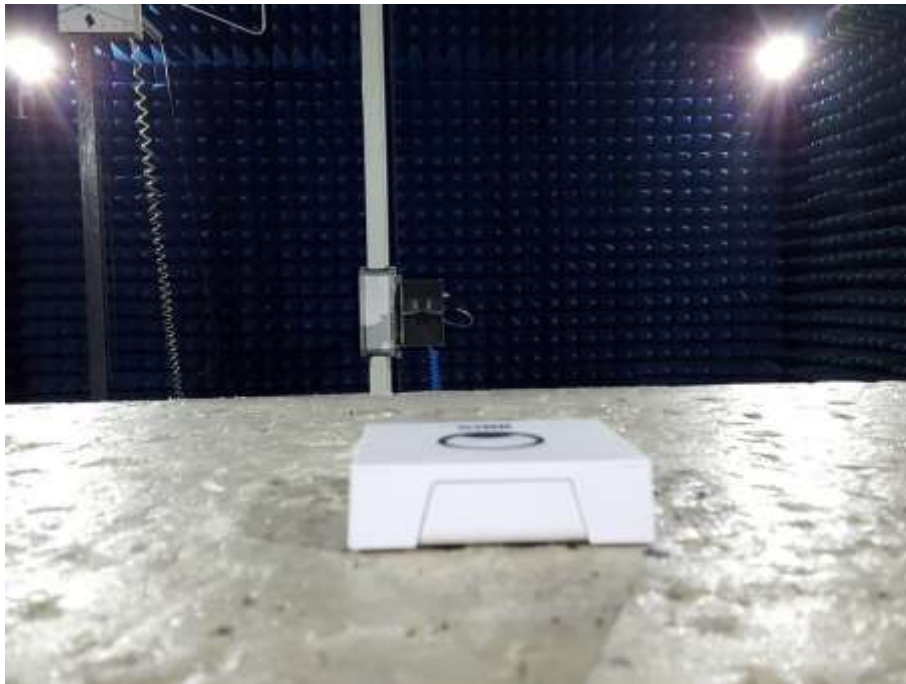
Photograph 3: Set-up for Radiated Spurious Emission (1GHz ~ 18GHz)
