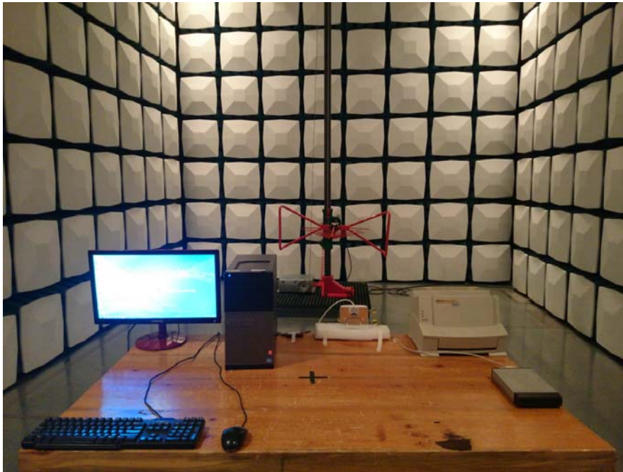
Radiated Emission - Front View (Below 1GHz) (Wall Mount Antenna)
