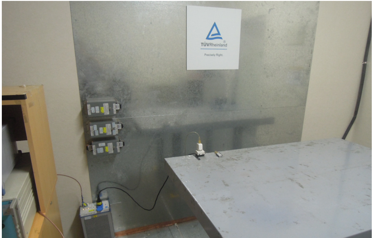
Photograph 8: Set-up for Mains Conducted testing Front
