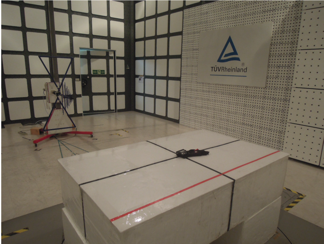
Photograph 3: Set-up for Radiated Emissions (Back View 2)
