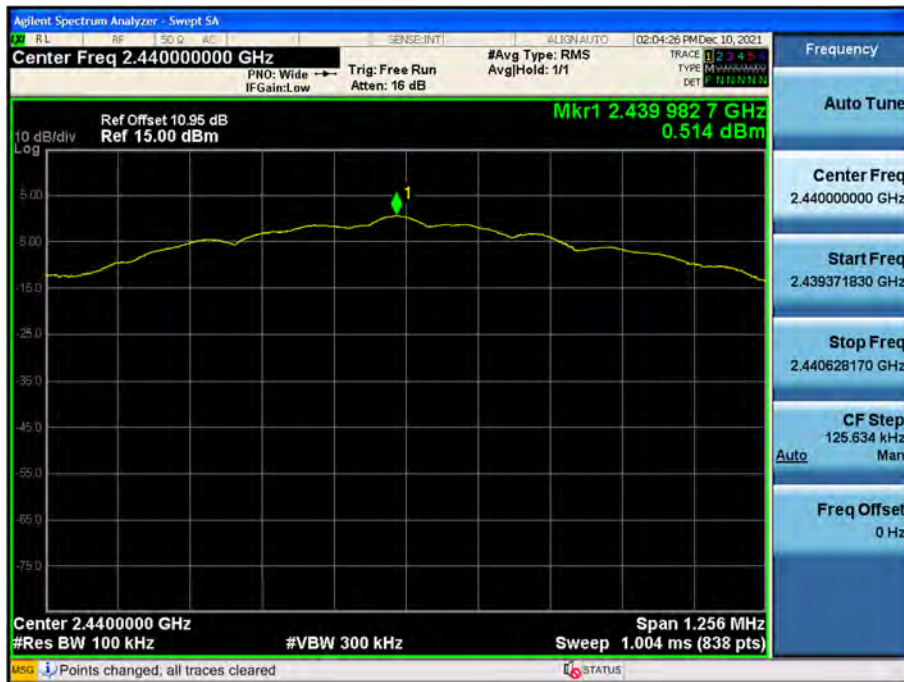
Power Spectral Density (Mid-CH 19)
