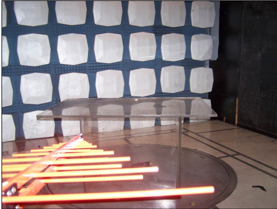
Photograph 3. Radiated Spurious Emissions, 30MHz-1GHz, Test Setup
