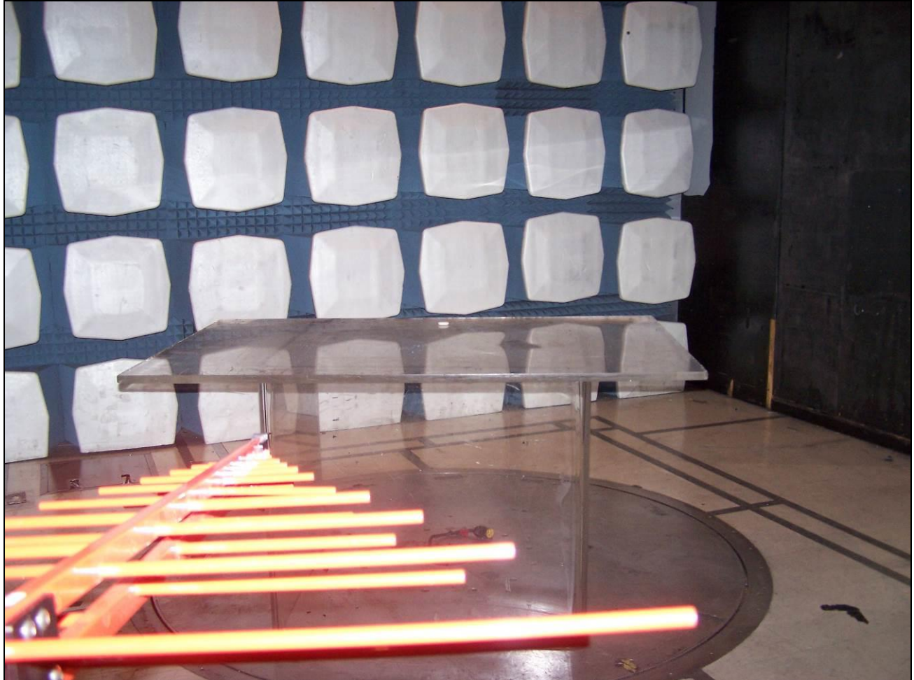
Photograph 2. Radiated Emissions, Test Setup
