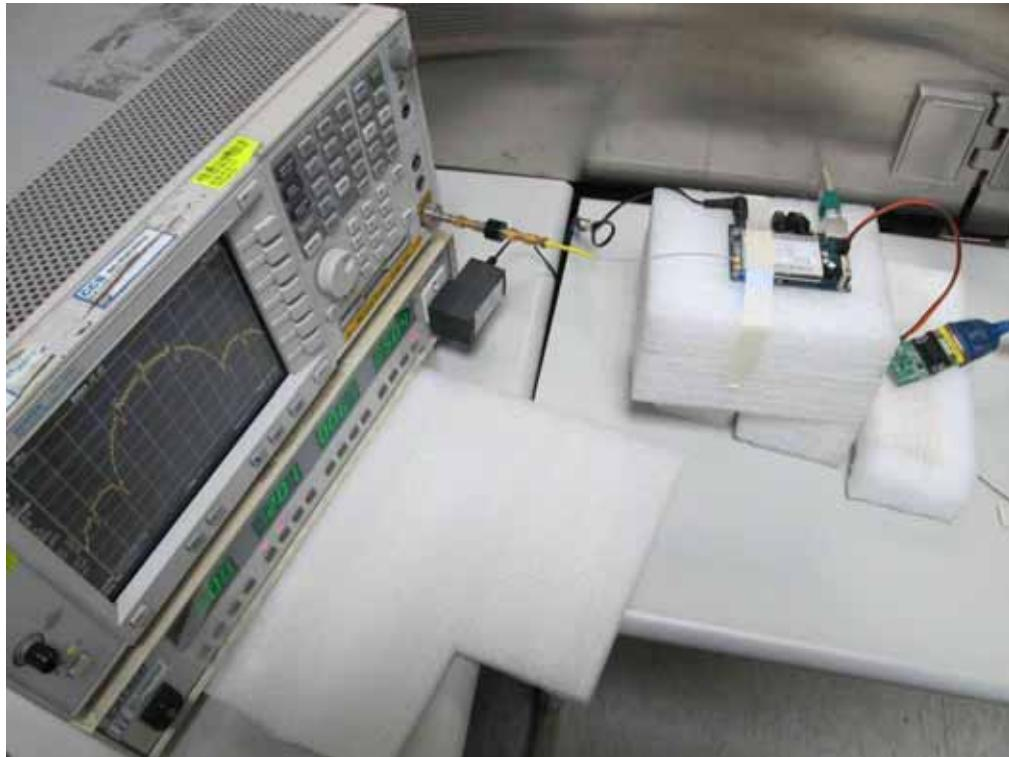
**CONDUCTED EMISSION SETUP****For Model SA9800-A1 Test**
