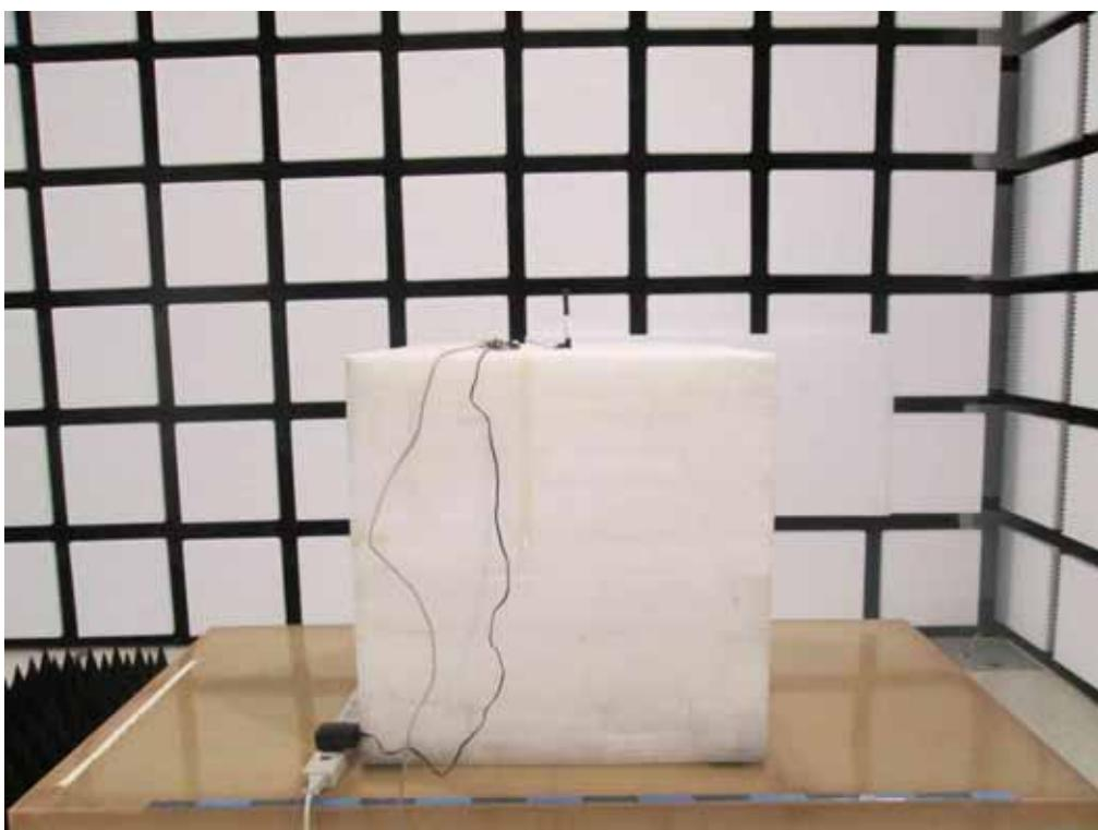
**ANTENNA PORT CONDUCTED RF MEASUREMENT SETUP****For Model SA9800-C1 Test**
