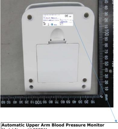
Automatic Upper Arm Blood Pressure Monitor Model No. : HL858DM Power: 1. DC 6V, AA "LR6" (1.5V) Alkaline Battery x 4 2. DC 5V 1A AC/DC Adapter: FranMar International, FRM06-S05-UU (optional)
