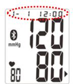
E. Without any operation for 1 minute, device automatically shuts off.
