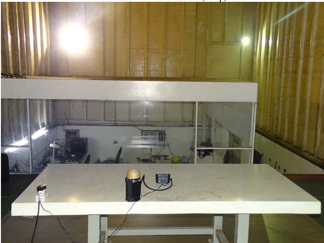
Back View of Radiated Test (Loop)
