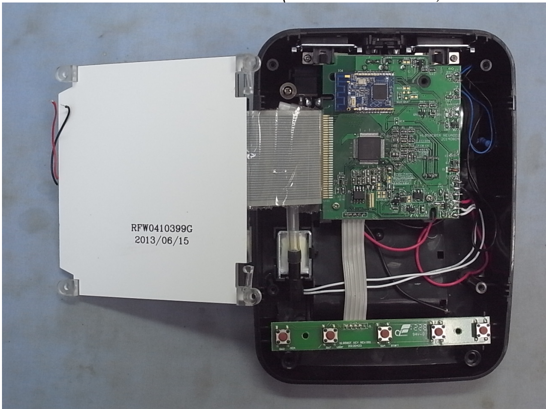
Figure 4 Internal View (Removed LCD Panel, LCA Panel/Back View)
