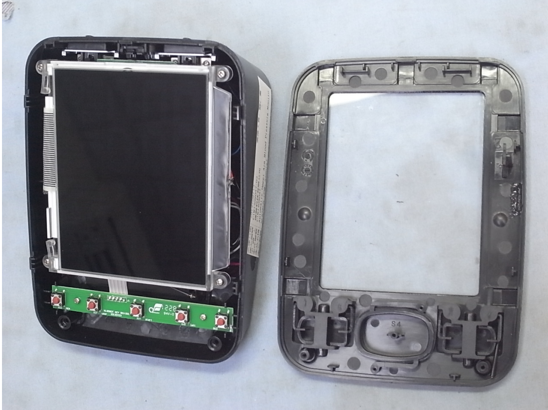
Figure 4 Internal View (Removed LCD Panel, LCA Panel/Back View)
