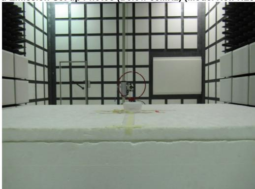
Radiated Emission Set up Photos (Below 1GHz)
