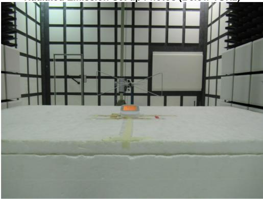
Radiated Emission Set up Photos (Front View)
