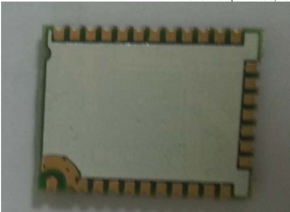
Figure 10 Internal View (BT Module, Back View)
