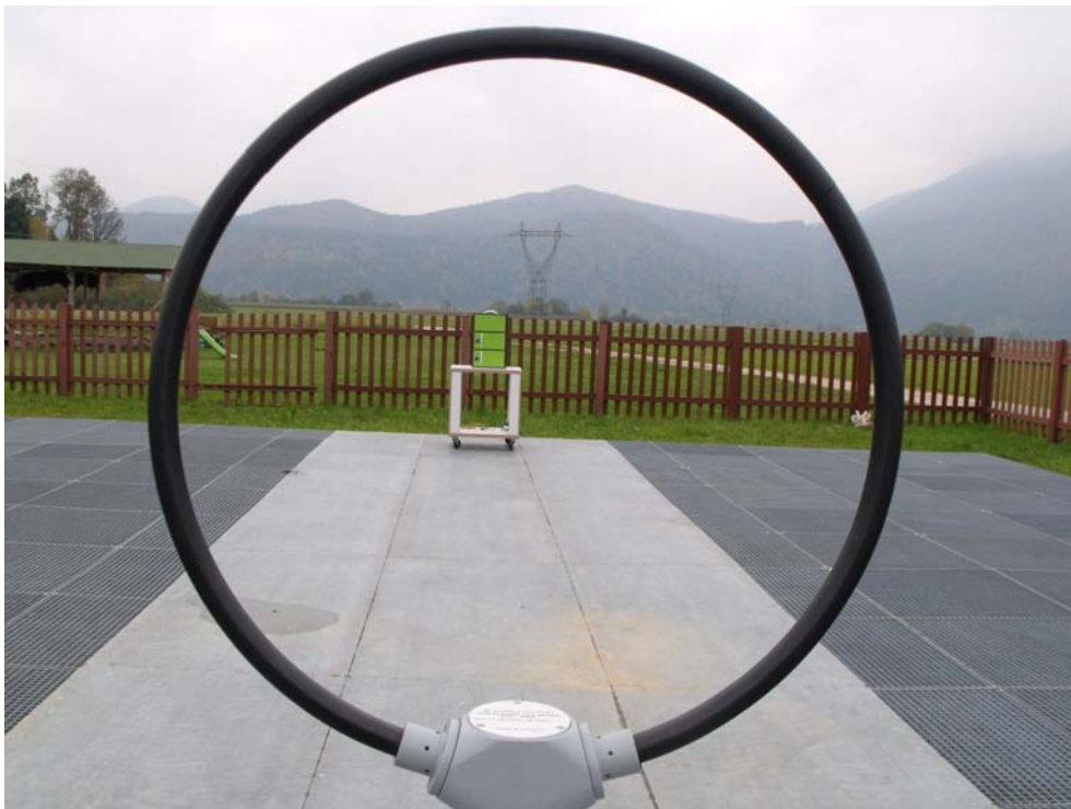
Figure 4: Radiated emission test – under 30 MHz on OATS
