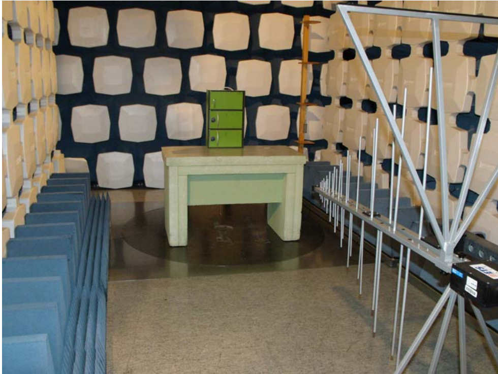
Figure 3: Radiated emission test – over 30 MHz
