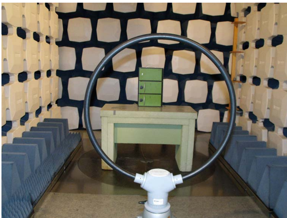
Figure 2: Radiated emission test – under 30 MHz
