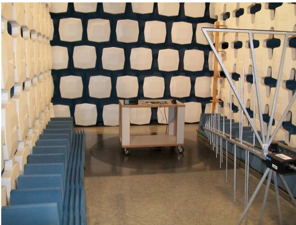
Figure 3: Radiated emission test – 30MHz to 1GHz
