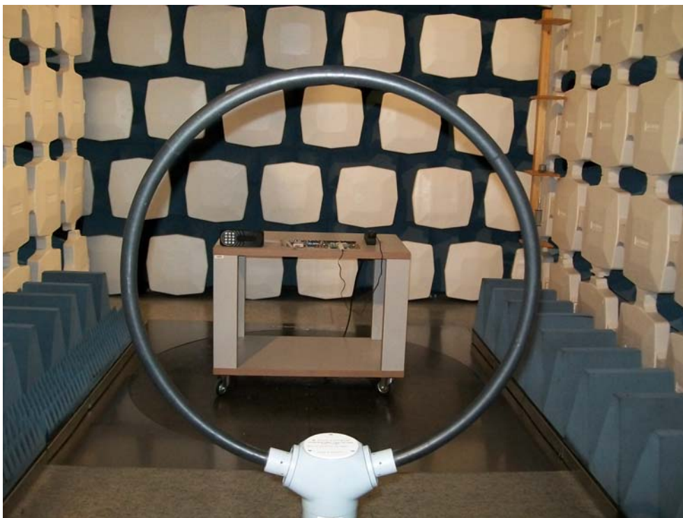
Figure 2: Radiated emission test – 9kHz to 30MHz
