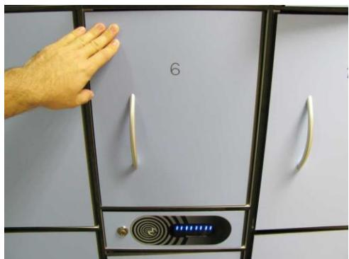
**STEP 1:** Close the locker door. Time countdown starts (vertical lines are displayed) on the Display and interrupted beep acoustic signal is activated.
