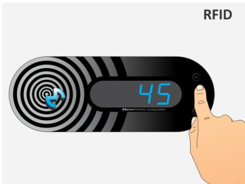
**STEP 1:** Select the desired locker number by pressing the 'up' key to increase or the 'down' key to decrease the currently selected locker number. Use the "Enter" key to confirm the unlocking of selected locker.
