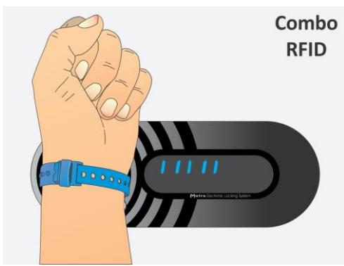
**STEP 2:** Approach the RFID media to the antenna field. Reading distance is 2 – 5 centimetres from the device surface. Hold the RFID media in the field for a few moments for device to read and process it.
