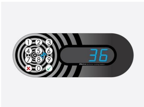
**STEP 5:** Locker number is displayed and corresponding locker is locked.
