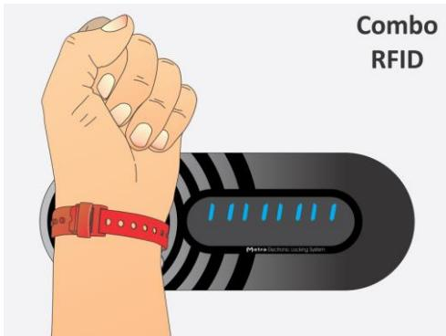
**STEP 2:** When the RFID media is accepted as a Multi key the multi locking mode is activated, countdown starts and vertical lines are displayed.
