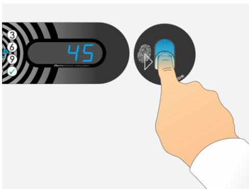
**STEP 3:** If the same finger is presented correctly corresponding locker is unlocked and opened. Short acoustic signal is also activated.
