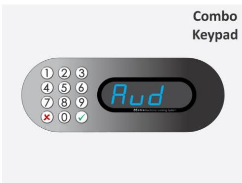
**STEP 4:** If correct Setup code was entered the Locker Controller turns to Basic Setup mode of operation. Sign “CodE” (if “Special Keys Mode” is set to “On-line” in Metra ELS/LCC NET software) or “Aud” (if “Special Keys Mode” is set to “Off-line” in Metra ELS/LCC NET software) as first parameter is displayed.
