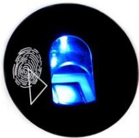
Fingerprint module allows users to lock/unlock the locker by presenting the finger to sensor. It offers higher comfort for users as they don't need to remember PIN code or carry around the RFID media. When fingerprint module is connected to ELS Locker Controller each user can freely choose whether he/she will lock the locker using fingerprint/PIN code/RFID media.
