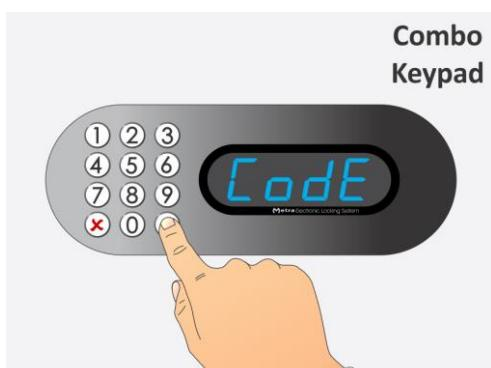
**STEP 2:** Sign "CodE" starts flashing beep acoustic signal is heard.
