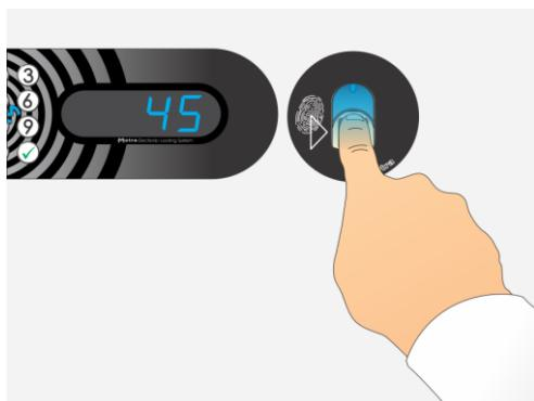
**STEP 3:** When the Fingerprint is accepted as a locker key the corresponding locker is locked and its number is displayed.
