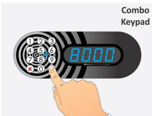
**STEP 1:** Enter group PIN code to start multiple unlocking procedure and press the
