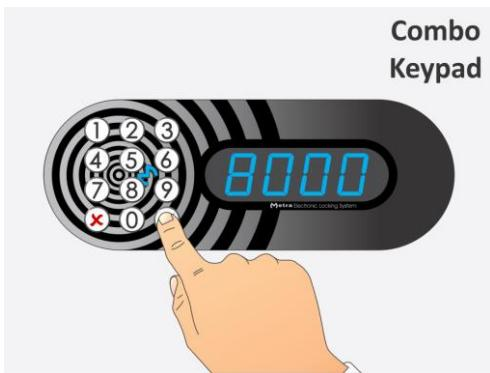
**STEP 1:** Enter group PIN code to start multiple unlocking procedure and press the ✓ key.
