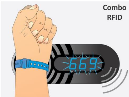
If the RFID media is presented and recognized as a locker key on different device the locker number is flashing on the display and interrupted acoustic signal is activated. Locker remains closed.
