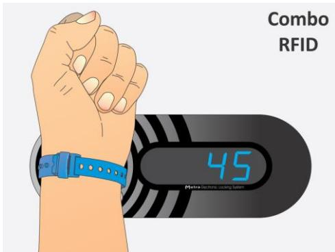
**STEP 2:** Display shows the locker number and the locker is unlocked when the RFID media is recognized as a locker key that previously locked that particular locker. Short acoustic signal is also activated.
