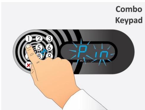
**STEP 2:** If **PIN code** was chosen sign “Pin” is flashing and beep acoustic signal is heard. Enter the PIN code that was used to lock multiple lockers and confirm it with ✓ key.
