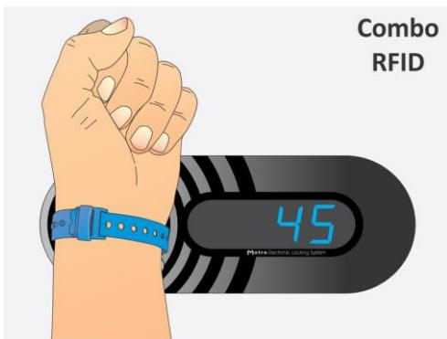
**STEP 3:** When the RFID media is accepted as a locker key the corresponding locker is locked and its number is displayed.
