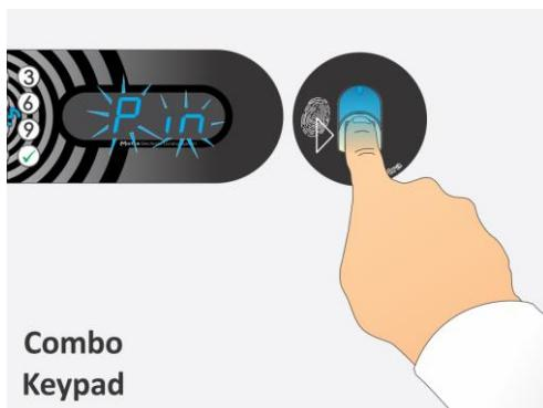
**NOTE:** If fingerprint is chosen than insert your finger in the Fingerprint module.
