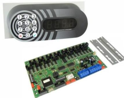
Metra Electronic Locking System (ELS) is primarily designed and used for locking lockers. Each ELS system has two basic components: Metra Locker Controller and Metra Display. Locker Controller drives and monitors up to 16 locks connected directly to the unit, with the possibility to add up to two Extension Modules for 8 additional Electronic Locks each. This enables configurations of 16, 24 or 32 locks, which makes the controller adoptable to many locker layout configurations.
