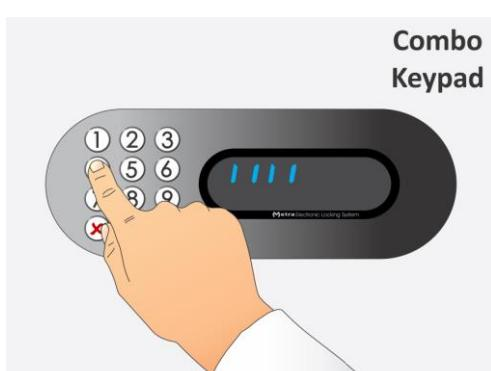
**STEP 3:** Type-in a Master code (up to 16 digits). Signs "I" are displayed for each entered digit. Confirm the Master code with the
