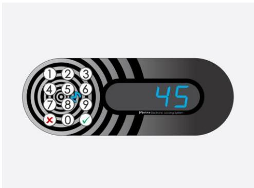
**STEP 3:** When all requested coins are inserted locker number is displayed and corresponding locker is unlocked and opened. Short acoustic signal is also activated.
