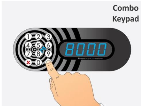
**STEP 1:** Enter group PIN code (number defined by "GrUP" parameter – from 8000 to 9999) to start multiple locking procedure and press the
