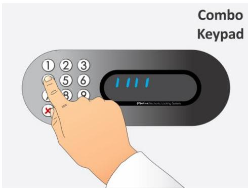
**STEP 3:** Type-in a Setup code (up to 16 digits). Signs “I” are displayed for each entered digit. Confirm the Setup code with the
