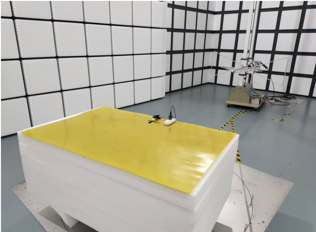
Photo of Radiated Emission Measurement (Above 1G)
