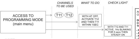
ACCESS TO MAIN MENU CONFIRMED, CHECK LIGHT ON STEADY. TX SENDS NO COMMANDS.
