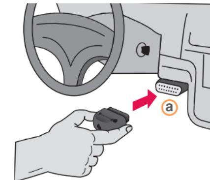
If unable to locate your vehicle manual, the SensorSafe Application may contain information regarding the location of the 16PIN OBDII port for your vehicle
