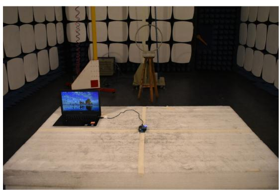
3. Radiated emission (9KHz-30MHz)
