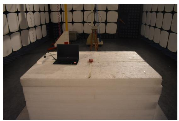
3. Radiated emission (9KHz-30MHz)
