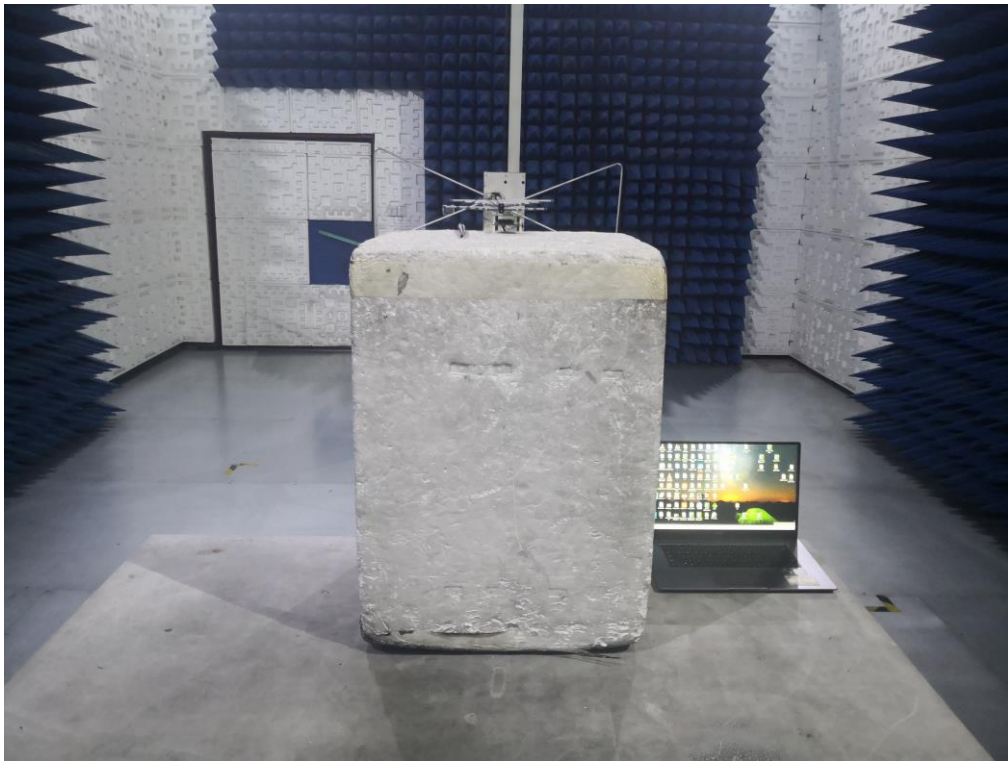
RADIATED EMISSION TEST SETUP ABOVE 1GHz
