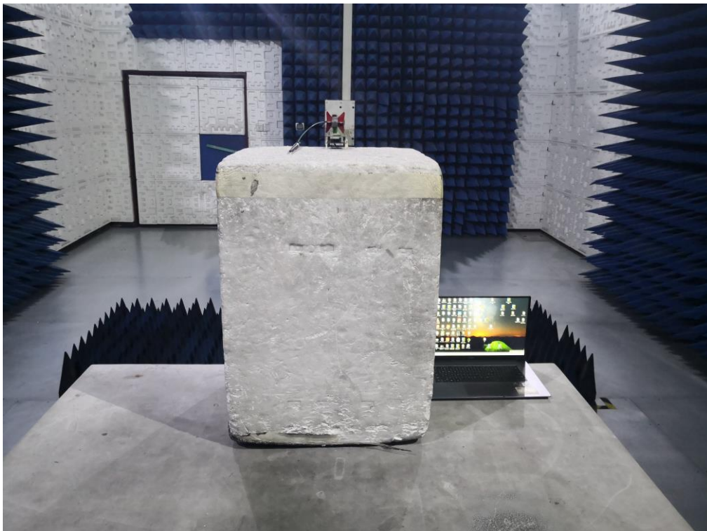
RADIATED EMISSION TEST SETUP ABOVE 1GHz
