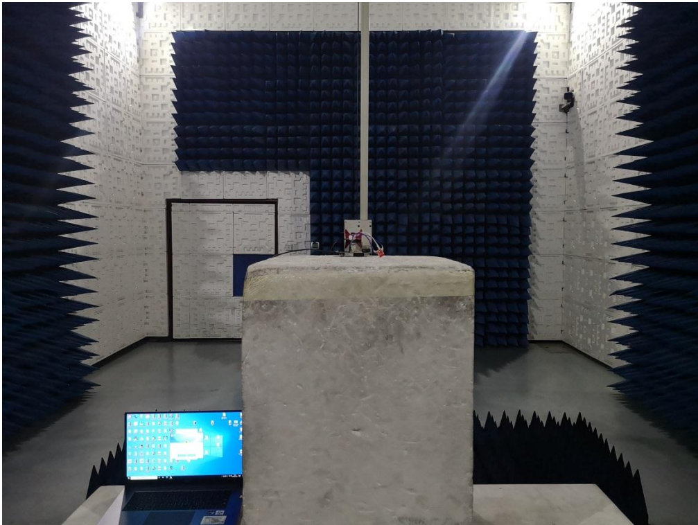
RADIATED EMISSION TEST SETUP ABOVE 1GHZ
