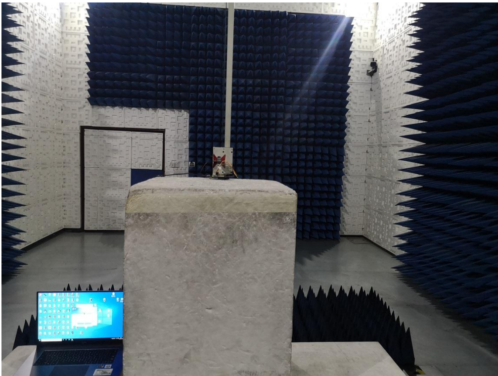
RADIATED EMISSION TEST SETUP ABOVE 1GHZ
