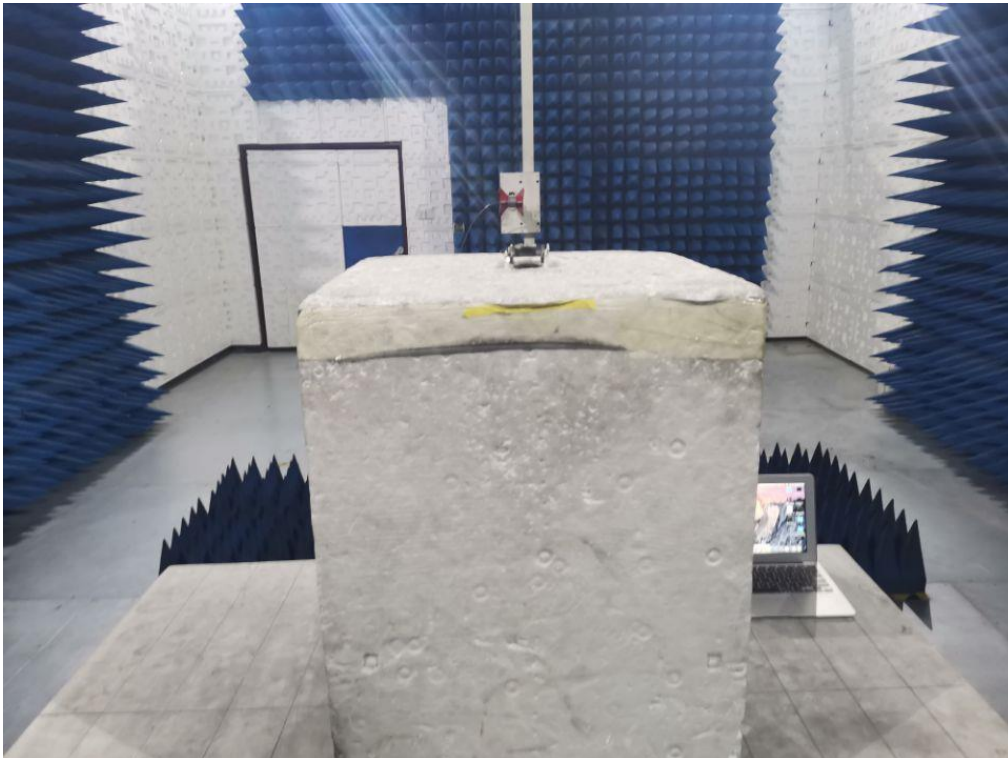
RADIATED EMISSION TEST SETUP ABOVE 1GHZ
