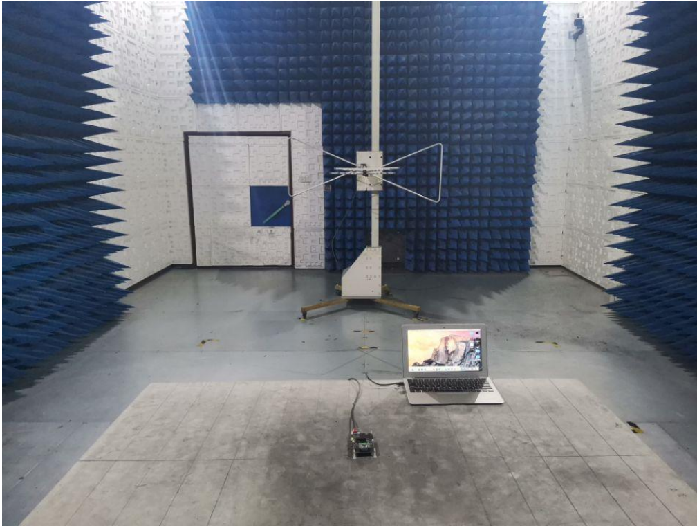
RADIATED EMISSION TEST SETUP ABOVE 1GHZ
