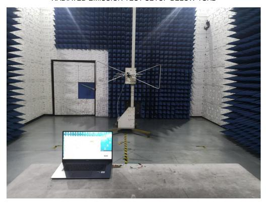
RADIATED EMISSION TEST SETUP ABOVE 1GHz
