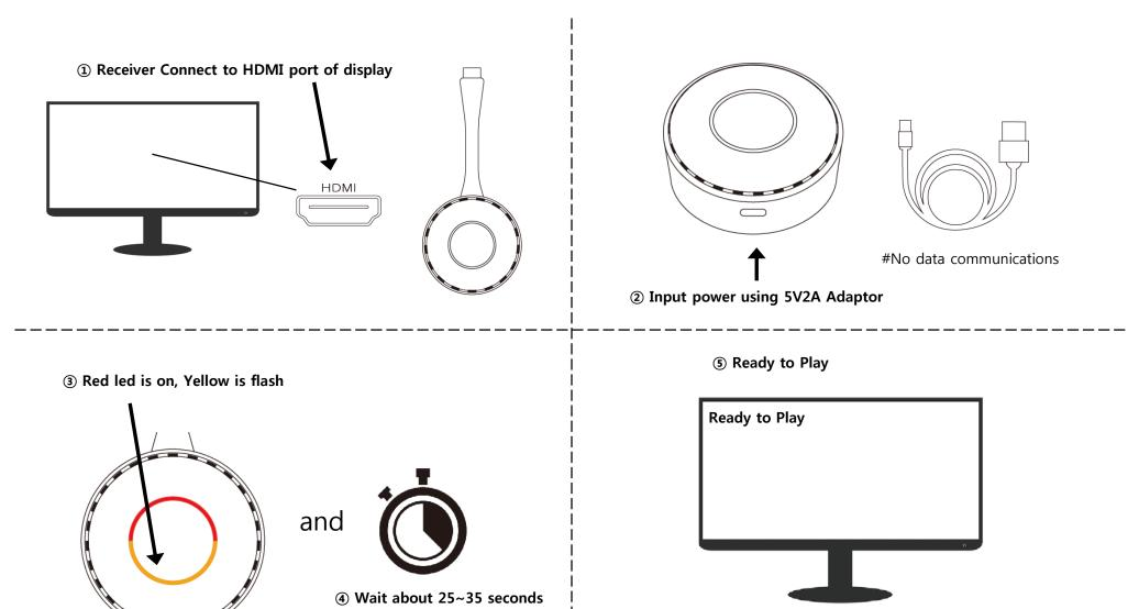
2. Transmitter installation and synchronize to Receiver
