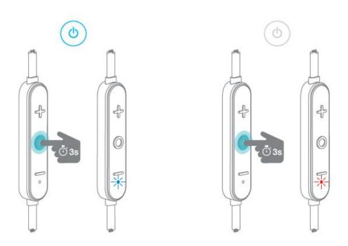
To power on your BE Sport4, press Power/Function button for about 4 seconds until the LED indicator flashes blue and you hear the "Power on" when voice prompt is activated or a beep if the voice prompt is not used. *NOTE:*
