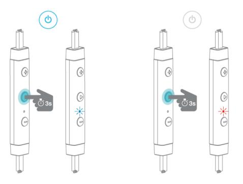
To power on your BE6i, press Power/Function button for about 3 seconds until the LED indicator flashes blue and you hear the "Power on" when voice prompt is activated or a beep if the voice prompt is not used. *NOTE:*
