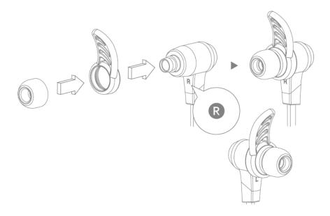
To ensure a secure and comfortable fit when wearing your BE6i:
