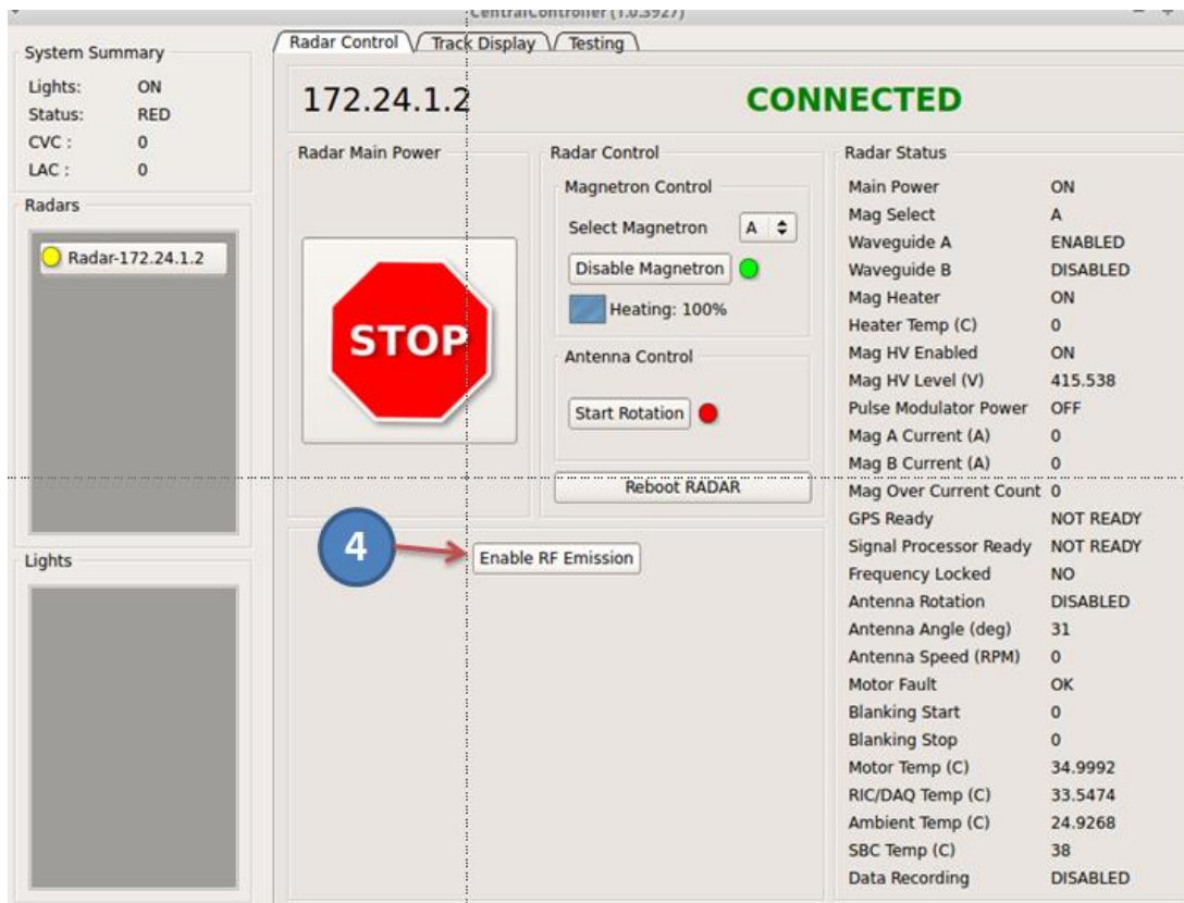
Figure 10. Radar Control GUI showing “Enable RF Emission” feature.
