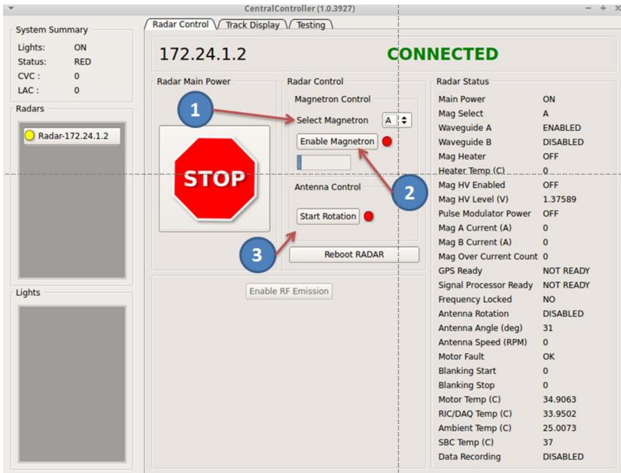
Figure 9. Radar Control GUI showing Magnetron Select feature.
