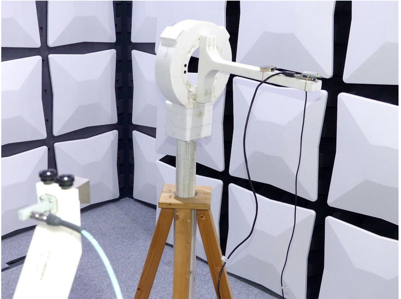
Photo 5: Test setup for radiated measurements (Enclosure, fully-anechoic chamber, 26-40 GHz intentional radiator §15, ANSI C63.10)
