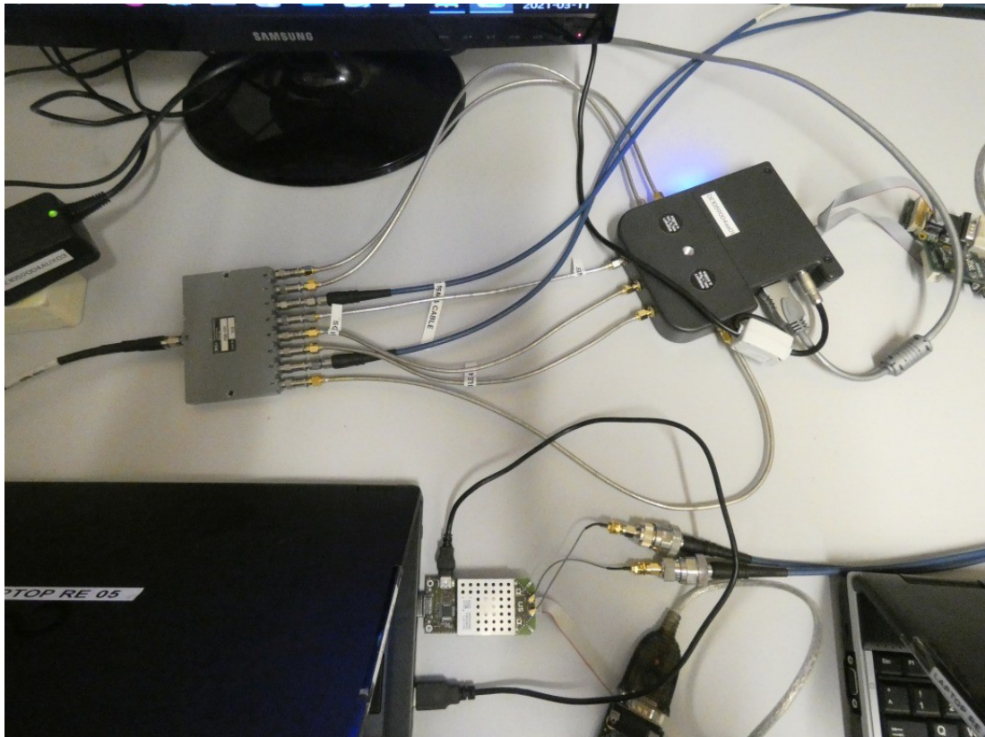
Photo 3: Test setup for conducted DFS measurements EUT detail
