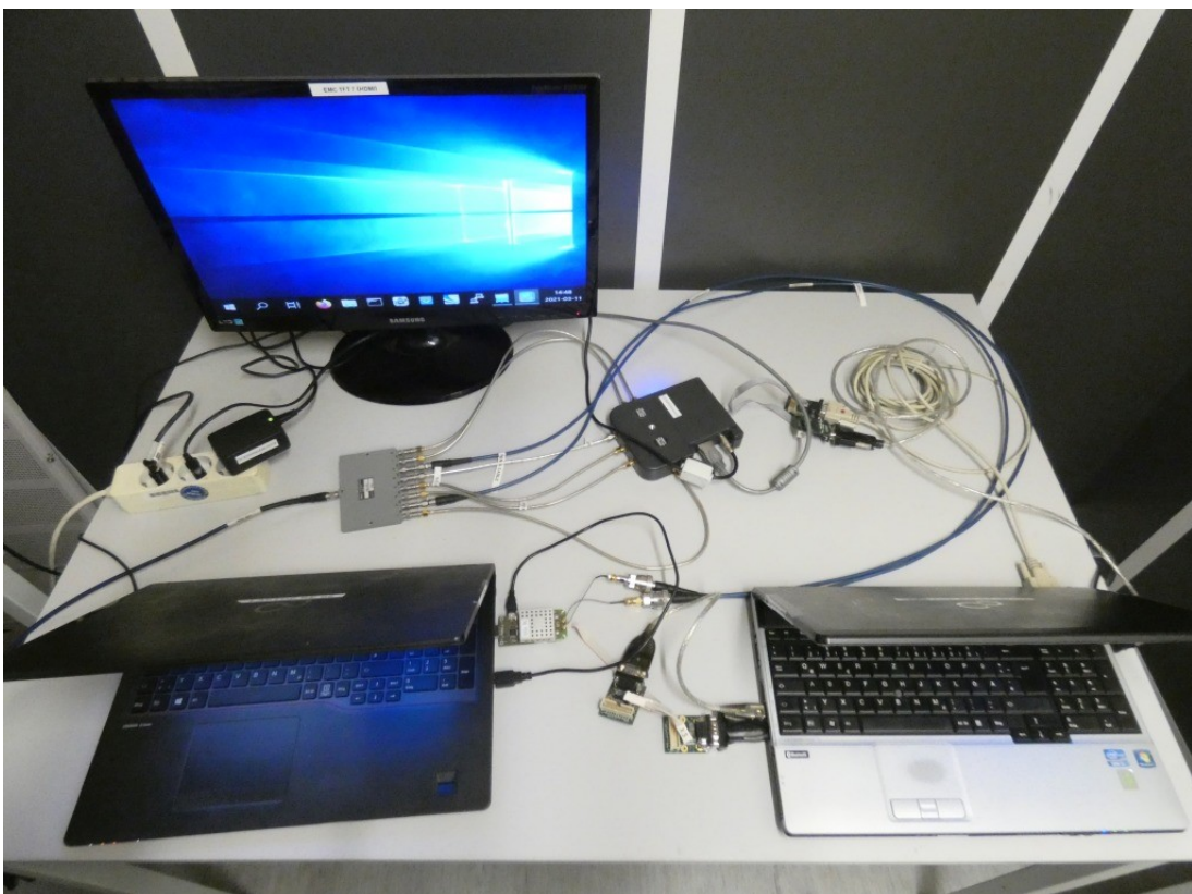
Photo 2: Test setup for conducted DFS measurements
