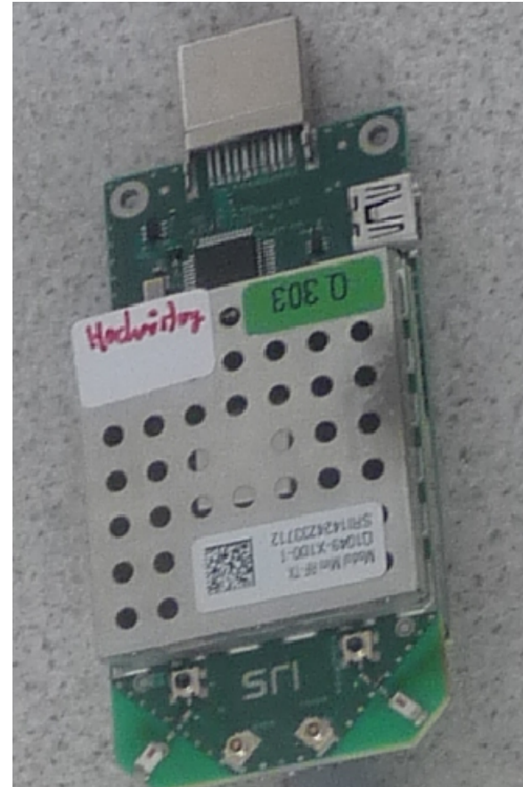
Q1049 RF Board Top with shield and installed
