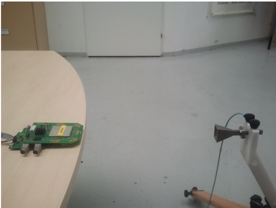
Photo 5: Test setup for radiated measurements (26 - 40 GHz)
