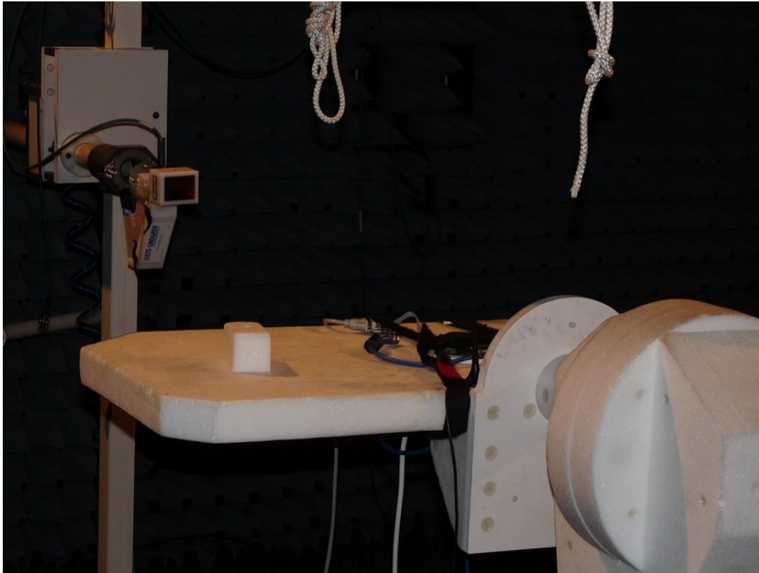
Photo 4: Test setup for radiated measurements (15 - 26 GHz)
