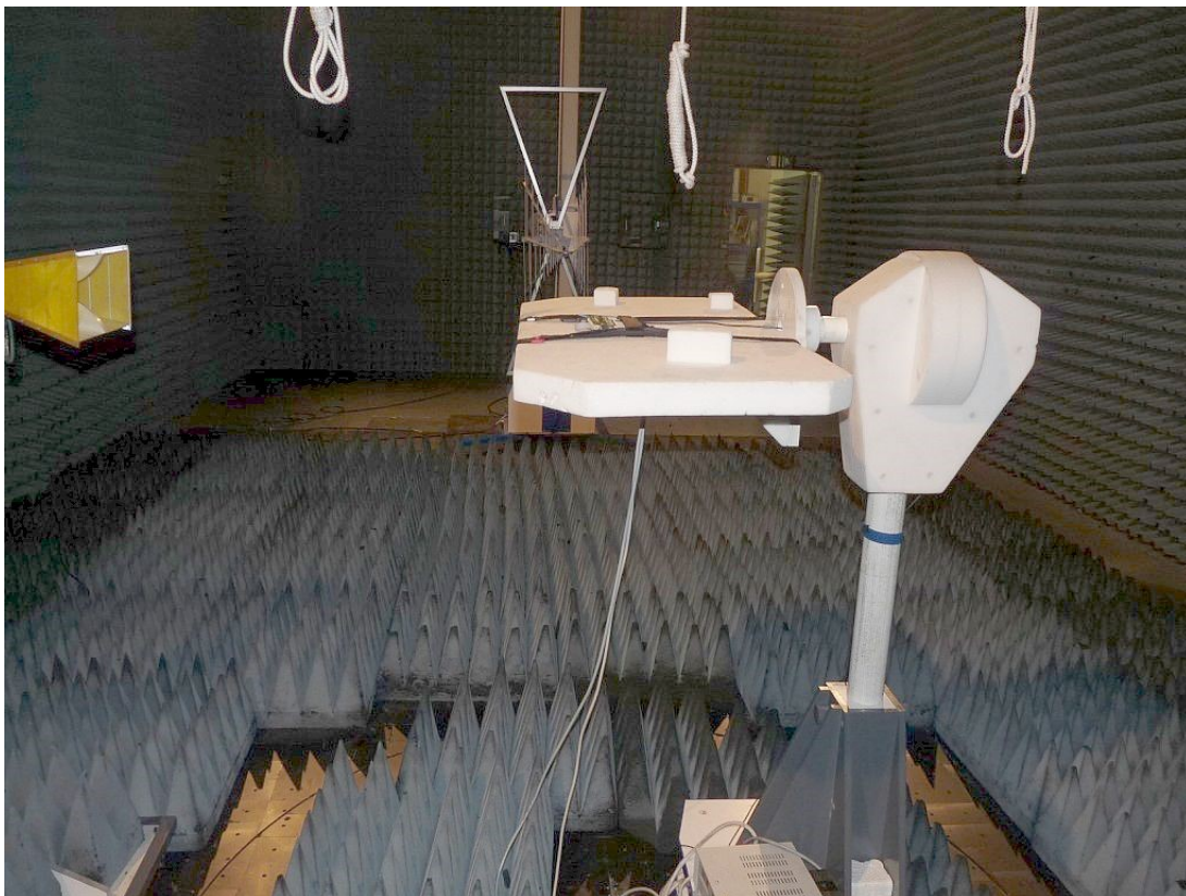
Photo 3: Test setup for radiated measurements (1 to 15 GHz)
