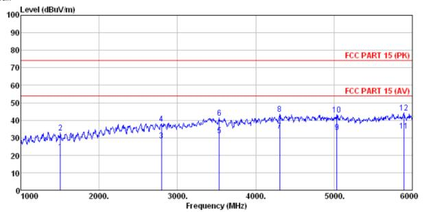
Site Condition : 3m chamber : FCC PART 15 (PK) 3m BBHA9120D ANT(>1GHZ) VERTICAL
