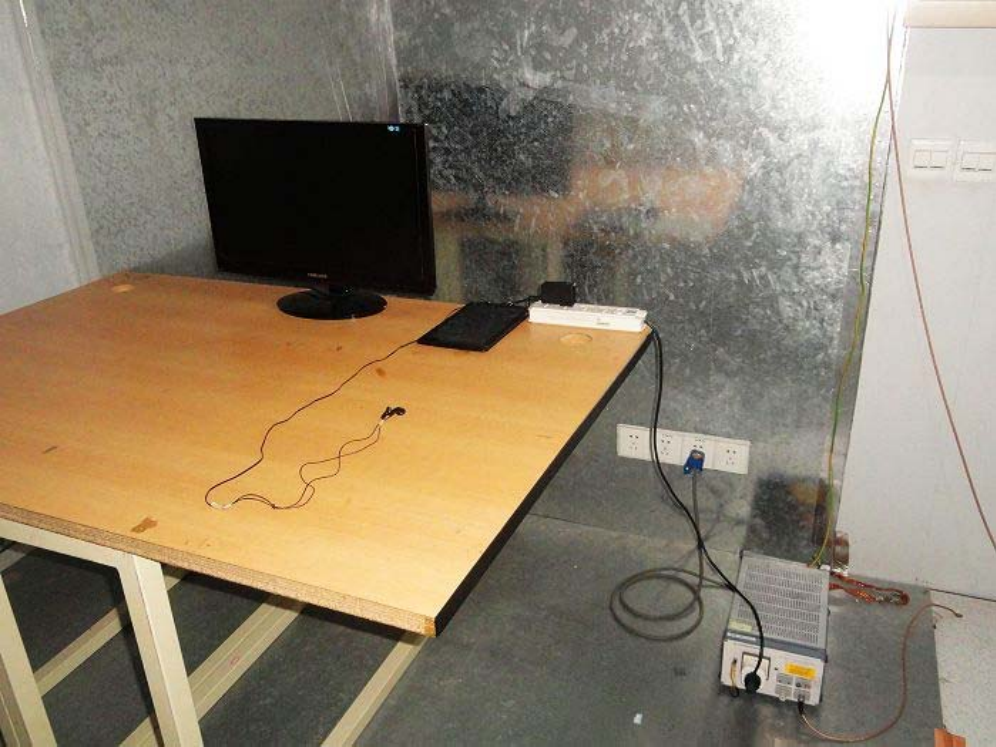
Conducted Emission Test Setup:
