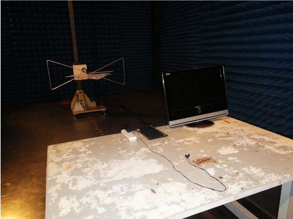
Radiated Emission Test Setup:
