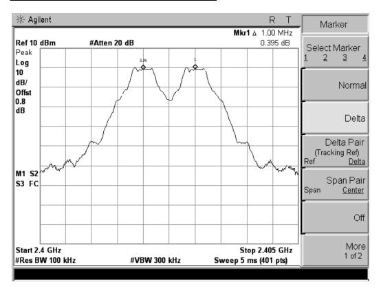
**Test Plot Of Frequency Separation (2Mbps)**
