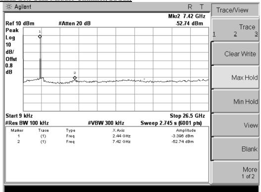
9KHz-26.5GHz High Channel(GFSK)
