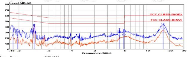
Env. Ins: EUT: M/N: Power Rating: Test Mode: Operator: Memo: Pol: 24\*/56% SoundBar HR-917 AC 120V/60Hz TX
