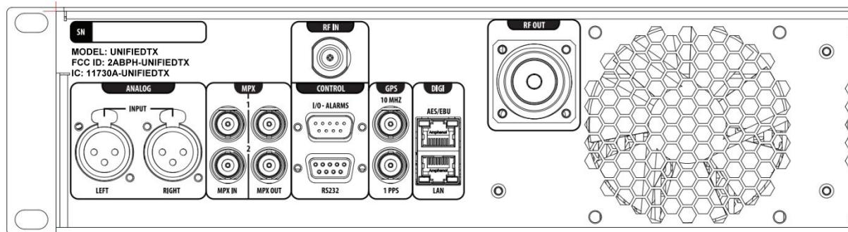
There are two options how the labels will be affixed to the unit. For standard production the label will be a part of non removable rear panel silk screen. For labelling the existing units a permanent sticker will be used.
